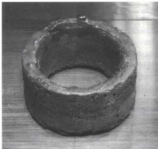
Plutonium-239 ring - The ring shape prevents chain reaction.
